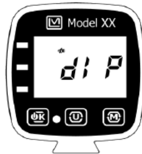
Figure 7.3: Setup - DIP switch protection enabled.
