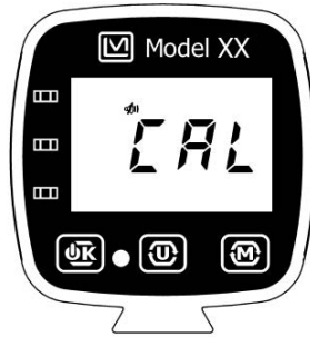
Figure 6.4: Fault - Calibration Expired.
