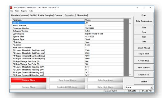
The Parameters tab displays all parameter settings that were used during the current record.
