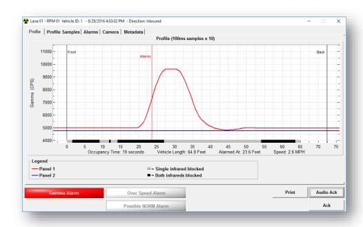
The Alarm window is automatically displayed and an alarm report is printed when a gamma alarm or over-speed alarm occurs. The alarm window is grouped into five tabs, each representing a different aspect of the alarm. The bottom of the alarm popup displays the gamma alarm status, over-speed alarm status, and the direction, date, and time of the occupancy. A Print button allows
