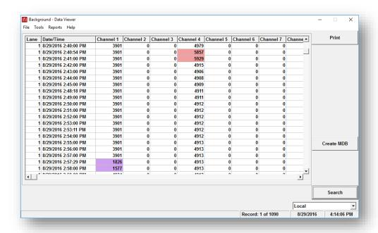
The main screen consists of a grid displaying the background readings recorded for all active RPMs when viewing background data. High background readings are colored with red, while low background readings are colored in purple.
