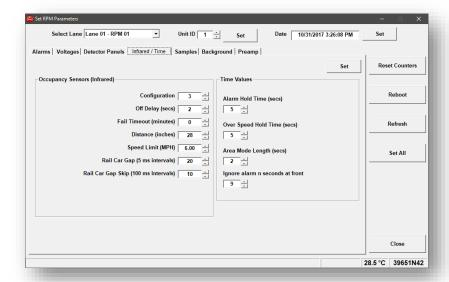
**Occupancy Sensor Configuration:** Sets the number of active infrared sensors. A setting of 1 enables only infrared sensor 1, a setting of 2 enables only infrared sensor 2, and a setting of 3 enables both infrared sensors. This allows the RPM to continue functioning if an infrared sensor has failed.
