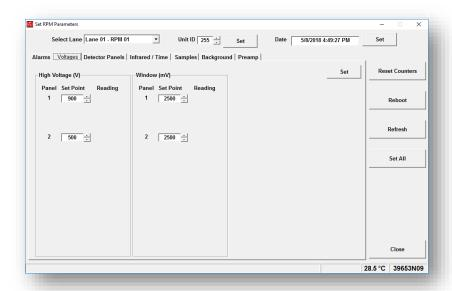
**High Voltage:** Sets the high voltage set point for each panel. Refer to the RPM calibration procedure for information on how to set these values properly. After changing the high voltage, the RPM should be rebooted.
