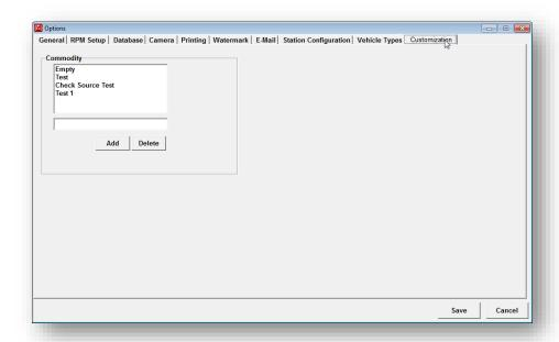
The Customization tab allows certain options to be modified with user-defined values. The default list of commodities can be set here allowing the user to pick from a list on the alarm and Data Viewer screens. Up to 20 user-defined commodities can be entered here.
