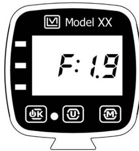
Figure 4.2: Firmware version display.
