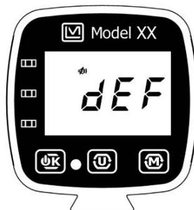
Figure 6.6: Fault - Defaults Loaded.
