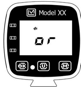
Figure 6.2: Fault - Over Range.
