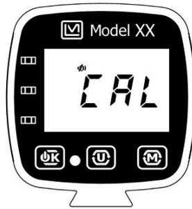
Figure 6.4: Fault - Calibration Expired.
