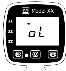
Figure 6.3: Fault - Overload.
