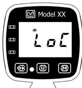
Figure 6.1: Fault - Loss of Counts.
