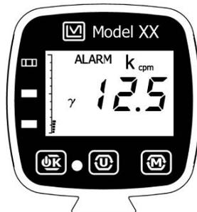
Figure 5.2: Alarm example in rate mode.
