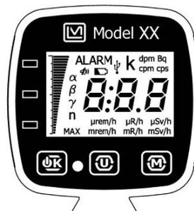
Figure 4.1: Startup display with all LCD segments shown.
