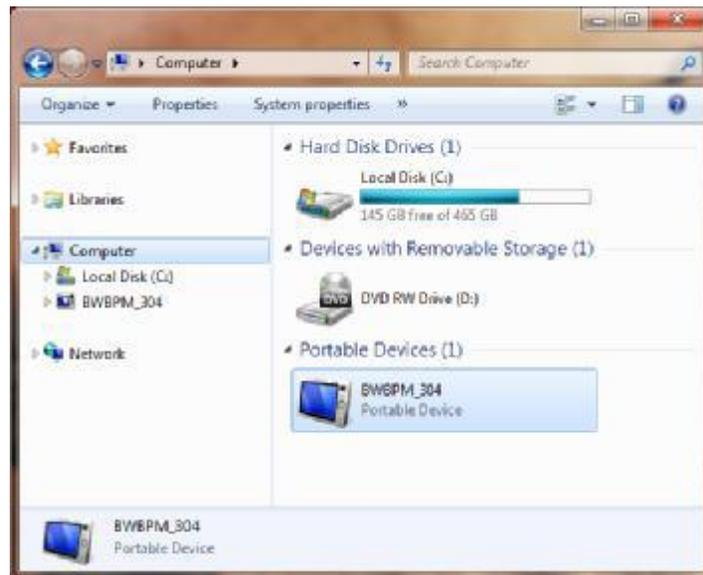
Double click the device icon in the File Explorer to open the files. The Bladewerx folder contains the log files on the Model 334A SD Card.
