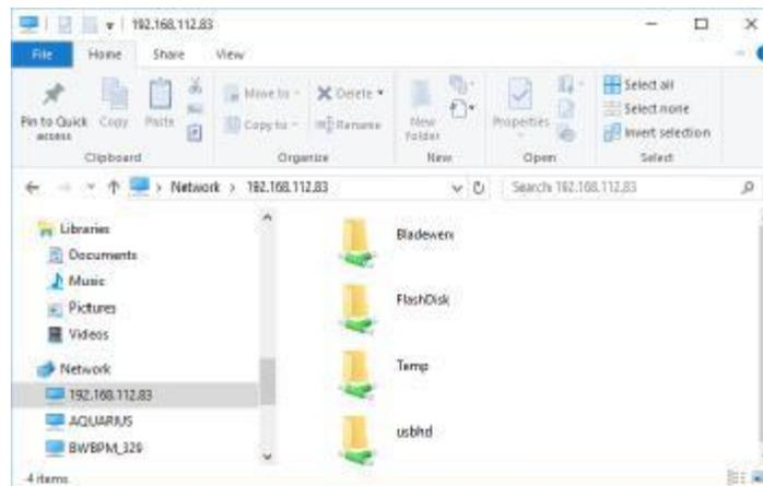
The Bladewerx folder contains the log files on the Model 334A SD Card.
