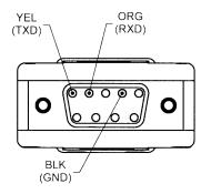
The left figure shows the RS-232 to USB cable for direct connection to a PC. The above figure depicts the 9-pin D connector portion of the cable up close.
