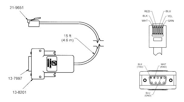
In the above, top-right figure, the phone plug is shown up close. The lower-right figure above is the 9-pin D connector portion of the cable depicted up close.
