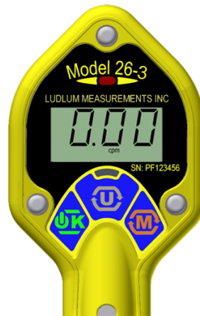
Figure 2.3: Detector Failure display (shown for cpm); will also flash.
