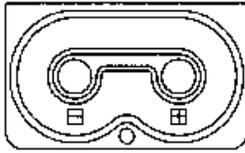
Install two "D" size batteries in the compartment. Note the (+) and (-) marks inside the battery door. Match the battery polarity to these marks. Close the battery box lid.
