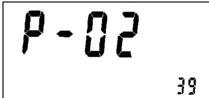
The LCD then displays the firmware number in the format "P-XX YY." The "XX" is the firmware number, and the "YY" is the firmware version. (The figure to the left is for example only; to illustrate location of display.)
