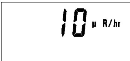
Check for a proper background reading:
