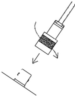
Connect a detector to the Model 2241 by using the cable provided; firmly pushing the connectors together while twisting clockwise until the connector latches (one-quarter turn). The diagram to the left illustrates how this is done.
