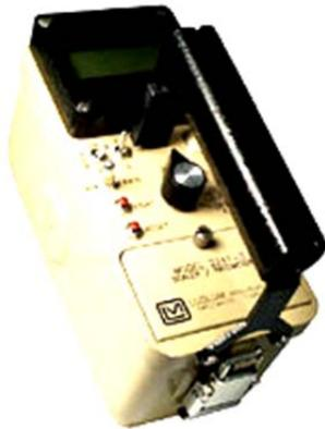
The Model 2241 is a portable microprocessor-based digital scaler/ratemeter designed for use with scintillation, Geiger-Mueller (GM), and proportional type detectors to measure ionizing radiation. Data is presented on a four-digit (six digits in the Scaler mode) Liquid Crystal Display (LCD) with moving decimal point. A three-position switch labeled OFF/RATEMETER/SCALER selects the desired operating mode for the instrument.
