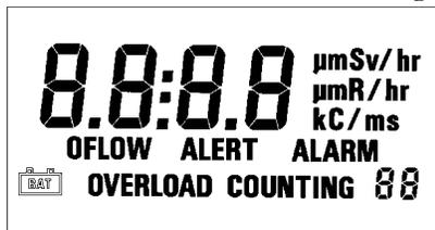
OVERFLOW when in the scaler counting mode (equivalent to a six-digit scaler) or exponential power when in the parameter setup mode. The upper right corner of the LCD displays units and multiplier(s) - R/hr, mR/hr, or  $\mu$ R/hr; Sv/h, mSv/h or  $\mu$ Sv/h; C/m, kC/m, C/s or kC/s. The bottom part of the readout displays the ALARM, ALERT, OFLOW, OVERLOAD annunciators and the low battery icon. COUNTING indicates that the scaler mode has been initiated and is in the counting process.
