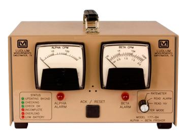
The radiation level is displayed on two analog meters. The Alpha meter dial indicates 0-1000 cpm on a three-decade log scale. The Beta meter dial indicates 0-100,000 cpm on a three-decade log scale. Each channel has its own distinguishable click-per-event audible tone. Beta events are a low pitch and alpha events are a high pitch. Beta clicks-per-event can be set at 1 per 1, 10, 100, or 1000.
