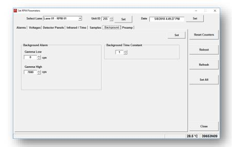
**Gamma/Neutron Low Set Point:** Sets the low background set point for all detector panels. If any panel's background reading drops below this value, a low background failure will occur. This can indicate a problem with a detector panel
