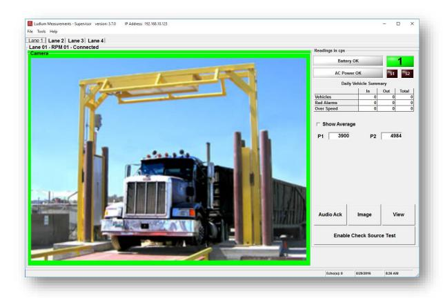
The main screen displays four tabs with each tab displaying the data for one lane. Each tab displays a camera image, battery and AC power status, infrared sensor indicators, and vehicle counts including number of radiation alarms and over-speed alarms, and the current background readings for each panel. There
