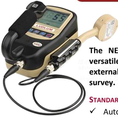
The NEW Model 3000 & 3001 series instruments are versatile, lightweight, & ergonomically-designed for use with external detectors for alpha, beta, and/or gamma radiation survey.
