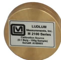
Calibrated 0.1 Bq/g (10 Bq) simulated <sup>60</sup>Co radiation source for use with the Model 2100 Sample Counter.
