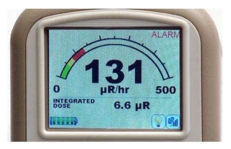
The Ludlum Model 9DP is equipped with a color LCD that improves the user's understanding of the instrument reading, functions, and operating status, as compared to other typical display technologies. The LCD utilizes a bit-mapped layout to afford an optimized arrangement of all of the data available.
