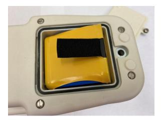
The location of the battery compartment is shown above. See the manual for instructions on battery removal.
