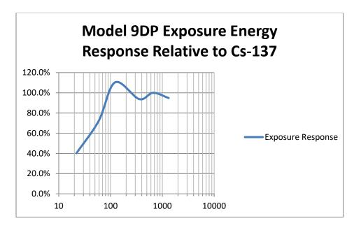
**Model 9DP\* Energy Response:** ambient equivalent dose or dose rate, flat within 20% from 40 keV to 1.3 MeV.
