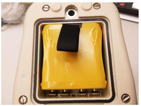
Be sure the instrument is shut down before removing the battery pack. The battery access door is located at the bottom of the instrument. The battery cover is held on by a single screw. Simply give the screw a quarter of a turn, and the door will pop up. Lift up the cover and remove it to fully expose the battery pack. Lift the battery pull-tab to lift out the battery pack. The battery pack snugly fits but comes out without much effort.
