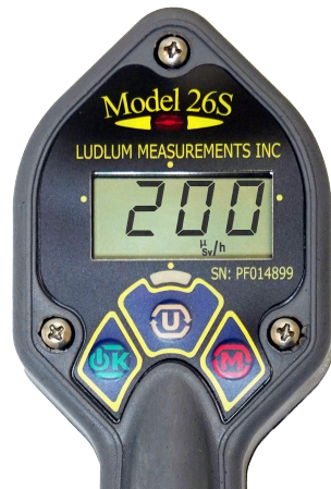
Figure 2.4: Detector Over Range (shown for \mu\text{Sv/h} ); will also flash.
