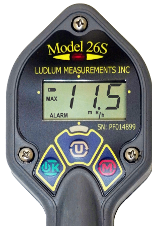
Figure 2.6: MAX Mode operation display with ALARM indicator and alarm LED.
