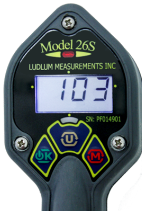
Figure 2.2: Firmware version display and ALARM LED check shown.
