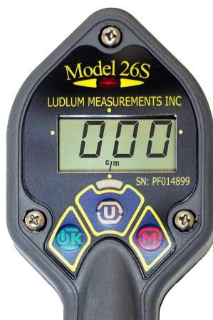
Figure 2.3: Detector Failure display (shown for c/m); will also flash.
