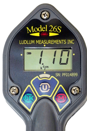
Figure 2.5: RATE mode display showing typical background radiation rate and the low-battery icon.
