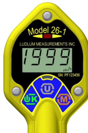
Figure 4: Detector Over Range (shown for \mu\text{Sv}/\text{h} ); will also flash.
