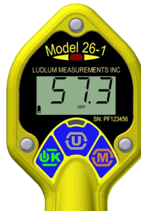
Figure 5: RATE mode display showing typical background radiation rate and the low-battery icon.
